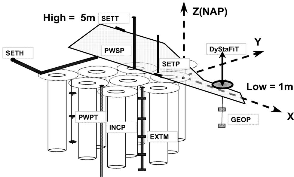
Figure 2. Instrumentation of test embankments
