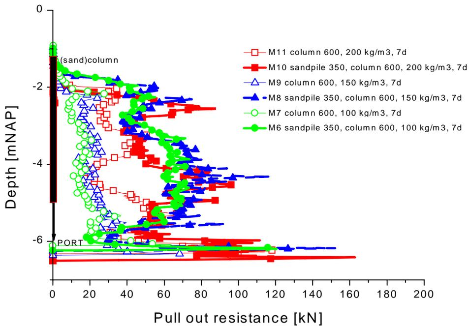
Figure 3. Inverted wing penetrometer results of single stabilized (sand) soil columns (HW0)
