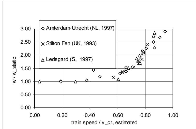
Figure 5. Scaled deflections (peak-to-peak) versus scaled train speed (dynamic amplification)
